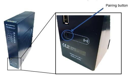
5.4. Press the pairing button of the wireless unit for a short period and select the TOOL number to be paired.
