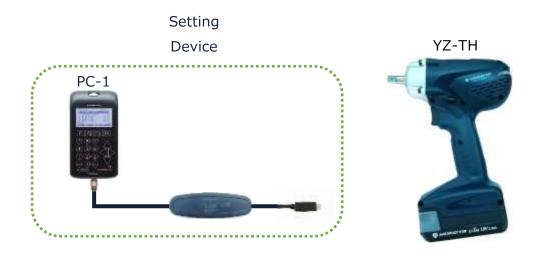
※[Setting device] described in this instruction manual, means programing console (PC-1) and special cable (CC-1) in connection.
