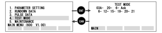
The test mode can enable the tool to rotate the main shaft after pulling the throttle lever as the usual rundown mode, and to tighten confirming the result after rundown judgement on the test mode screen. It is used for parameter setting and output adjustment.
