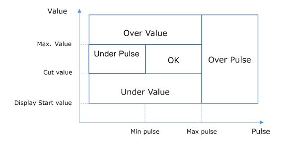
XValue: A guide value at which the tool will shutoff once it reaches during rundown
