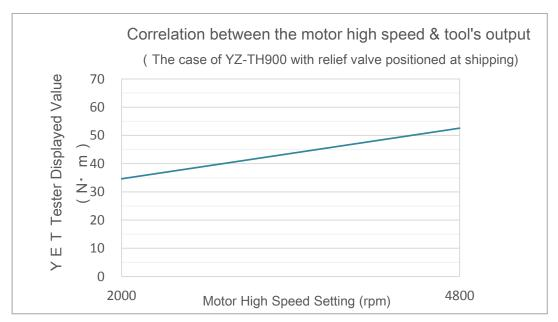
\*The above is one example of the tester displayed value of YZ-TH900 measured with our tester YET-1001C.
