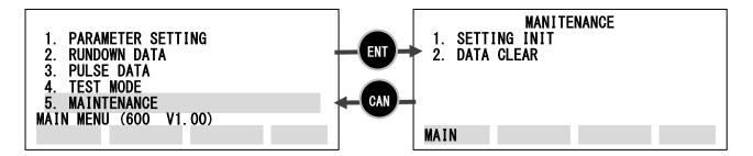
On the MAINTENANCE screen, select each item by up & down key and press enter key to conduct each function.
